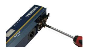
First, the track cleaning car must be unscrewed, then you can remove all the parts carefully. If you first remove the vacuum cleaner wheel with the provided tool (enclosed with the cleaning cart), the motor can be easily lifted off. In doing so, this empties the car so the circuit board can be removed.
